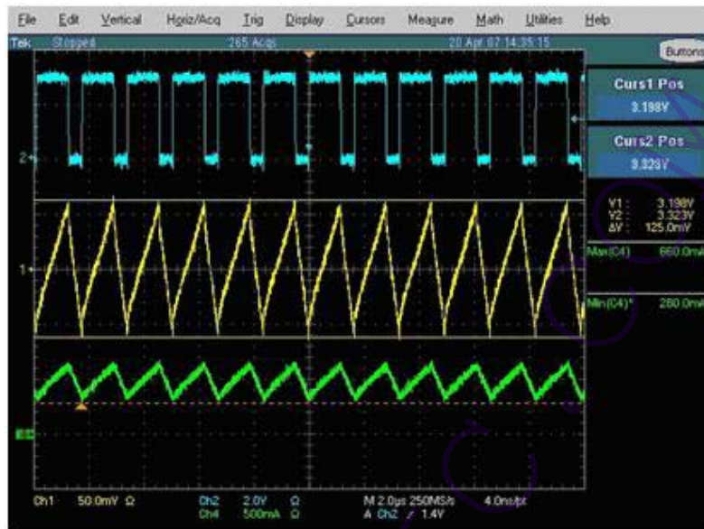
Figure 15. Electrolytic 100 \mu F (Ripple Too High)
