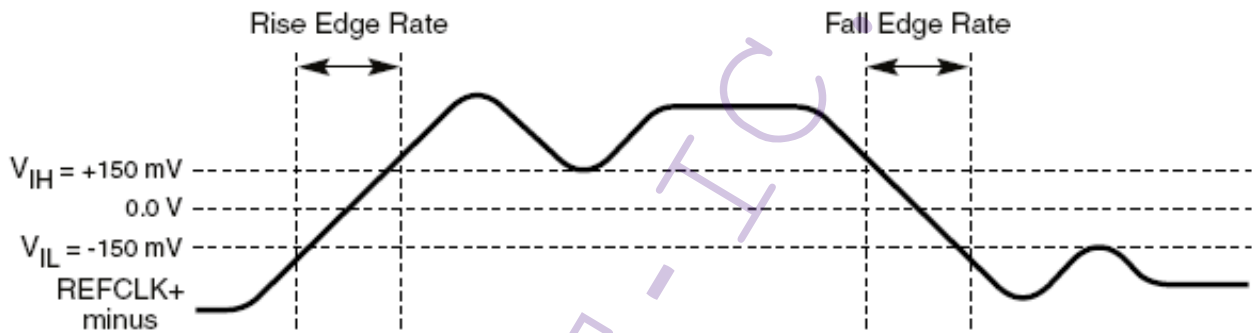
Figure 25. Differential Measurement Points for Rise and Fall Time
